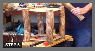
It is best to cut the largest branches for each corner first and then glue to the top and bottom pieces of plywood. Clamp diagonally to hold square shape while glue dries.
