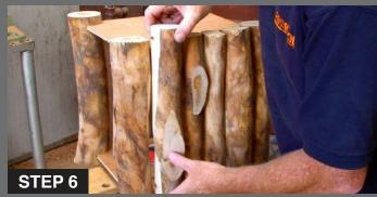
Now select and place the rest of the branches around the edges so that they nestle into each other. Then cut a slot for the top fit and place again to see if any excess wood needs to be shaved to make a close fit. With the top slot fitted to the top plywood, mark and cut the bottom slot. Use the turbo plane to shave and trim any excess wood from each piece before gluing. It is best at this stage to number each piece on the top.
