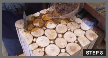
When your glue is dry you can start to plane the sides using the TURBOPlane so that you get a nice flat finish. Start by marking out a line in pencil on the top of your table showing where the plywood panel below as this will give you a guide where to plane. You can plane the sides up to 20mm from that line. Mix up either epoxy with woodchips or wood glue with woodchips and spread over the top of the table forcing the mixture down between the gaps to overflowing if necessary.
