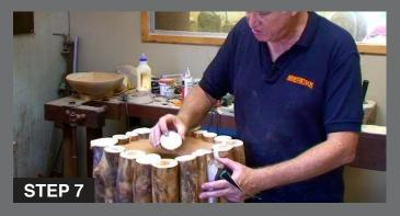
Once you have cut and shaved each piece to shape and are happy with the final shape you can glue each piece into place at both slots to the plywood. While the sides are drying you can cut some small pieces of approximately 20mm thick and start gluing them onto the top of the table including some very small rounds as well as large ones trying to fill in all of the gaps.
