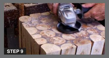
Once this is dry you can use the TURBOPlane to finish the top before sanding. Sand any sharp edges of the sides with the Contour Random Sander and finish off sanding the sides and the top of your table either by hand or using the Contour Random Sander.
