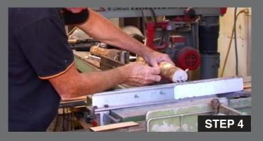
Place each branch onto the jig and mark where you want to make the slot cut on top. Then turn the branch over and set your saw to the required depth by running your branch in the jig against the blade of the saw before turning it on. Make sure your first cut is 20mm from the end of the branch and use an offcut to determine the width of cut.
