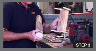
Make a small jig to hold branches for cutting slots by using a small piece of milled wood and screw or nail small pieces of V shaped board at each end. This will then give a stable base to cradle each branch and cut a slot.
