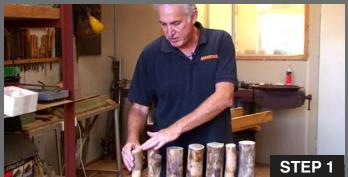
Grab a bunch of dried branches about 30mm – 50mm in diameter, enough to make up the perimeter of your table when layed side by side. Cut them to desired length (at the height of the table) plus approximately 10 mm to allow for planing the surface level . You can use any type of saw to cut these to length including a handsaw, bench or radial arm saw.
